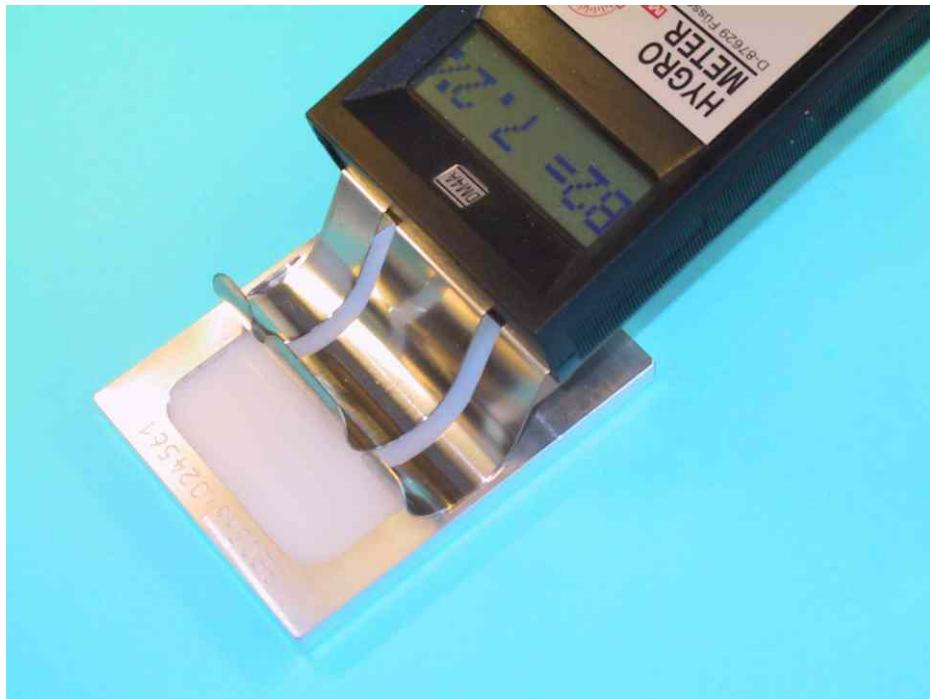
The test module PE305 can be used for testing and calibrating our capacitive moisture meters.
