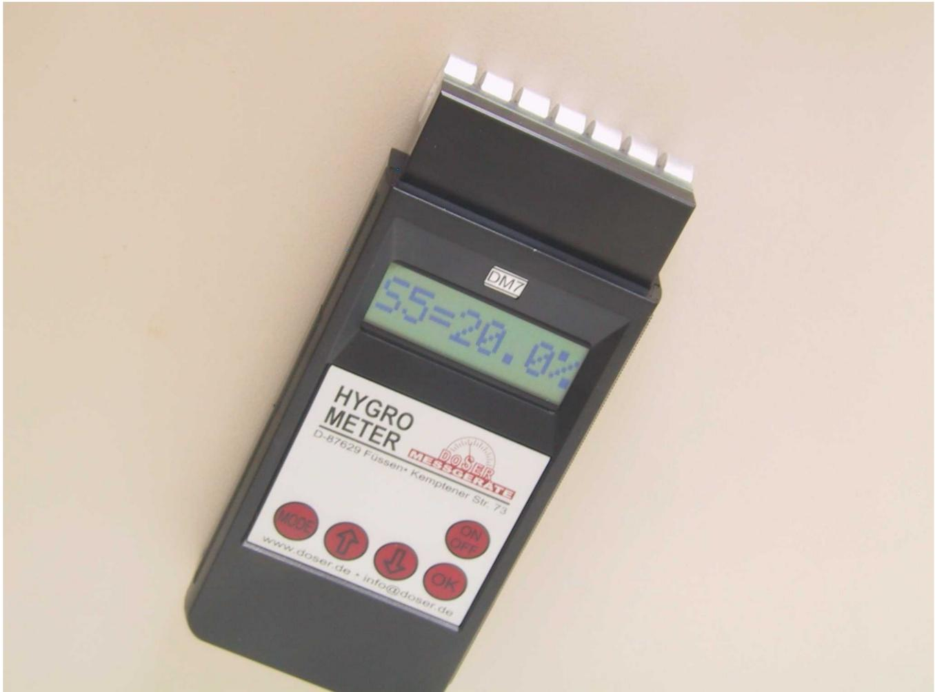
Moisture Meter type DM7 for veneers, corrugated boards, single card boards, cardboard pipes etc.
